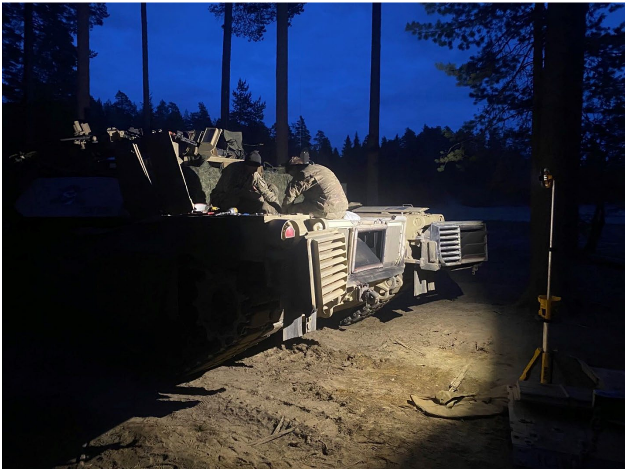
Figure 3. Mechanics from Assault Company, 1 st Battalion, 8 th Cavalry Regiment's field maintenance team conduct battle damage assessment repair on an M1A2 SEPv3 Abrams tank during Operation Lock, May 2023. (Army photo by 1LT Raven Parker, battalion unit public affairs representative)
